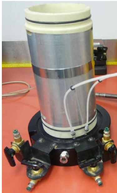
Figure 10. Split mold sit on pressure chamber base
