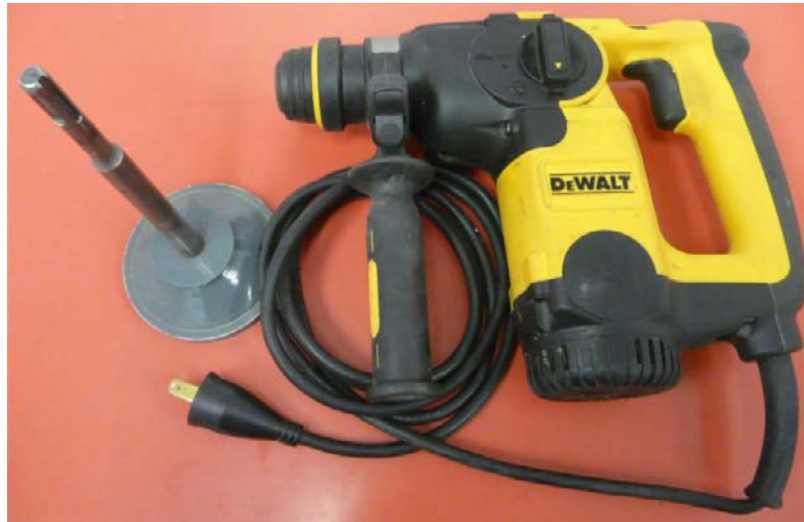
Figure 11. Compaction plate with rod and electric rotary hammer drill
