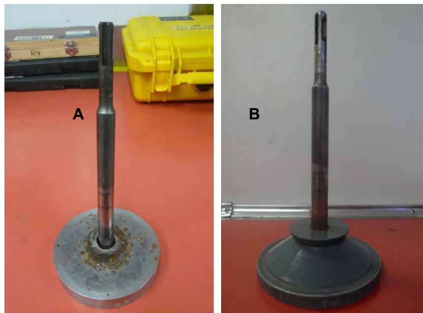
Figure 12. Compaction plate and rod: flat (A) and tapered (B)
