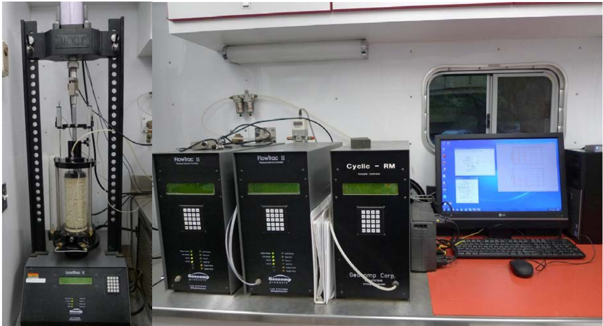
Figure 16. Triaxial pressure chamber, load unit, and computer used for permanent deformation and M_r tests.
